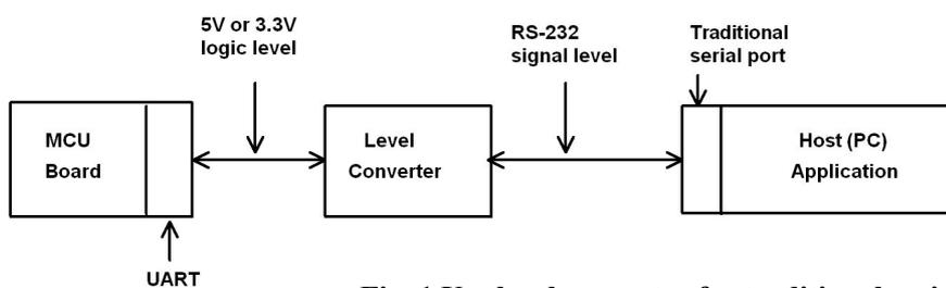
**Fig. 1 Use level converter for traditional serial port**
